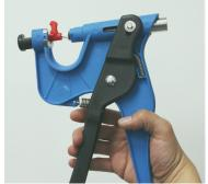
Rotate the black chamber to lock the punch into the device. Carefully squeeze the applicator handles together, guiding the punch tip into place if necessary. When the gun bolt rests flush against the red plastic clip, release the handle.
