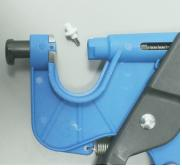
Reopen the chamber and remove the punch from the applicator. Check that sampling has been successful (red plunger is visible, sample is in fluid in punch). Remove the used cutter from the applicator by pulling the handles apart. Discard carefully as the cutter is very sharp.
