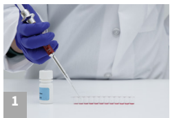
1 Remove 1 red mixing well for each sample plus 4 for controls. Remove equal number of clear antibody wells and place in well holder. Add 100 µL of conjugate to each red-marked mixing well.
