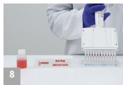
8 Transfer (using the 12-channel pipettor) 100 µL of Red Stop Solution from reagent boat into the antibody wells and mix by sliding back and forth on a flat surface.
