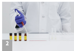
2 Add 100 µL of controls and extracted samples to the red-marked mixing well. Make sure the controls are in the correct order per the kit instructions.
