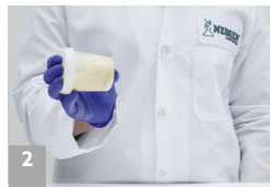
2 Add 50 mL distilled or deionized water and shake vigorously, once settled filter and collect filtrate
