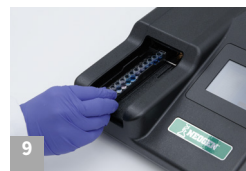
9 Wipe the bottom of the microwells with a dry cloth and read using a microwell reader with a 650 nm filter.
