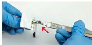
2. Slide handle up into slot on blade.
