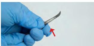
5. To remove blade from handle, push up on the base of the blade.
